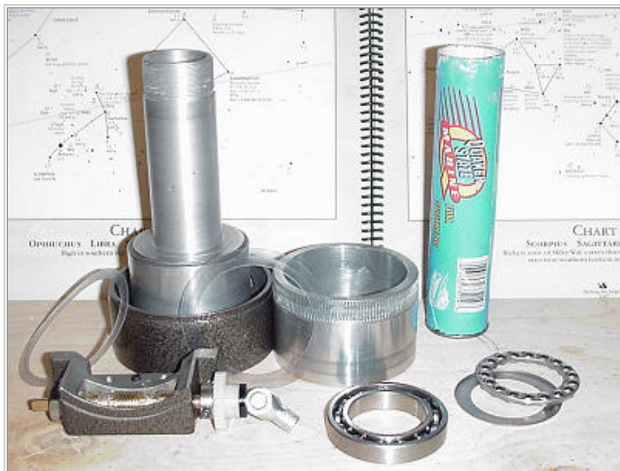
Internal RA components of the "new" CG-5, with ball bearings. Photo courtesy of Robert Burns
